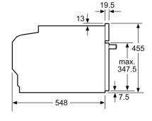
measurements in mm
