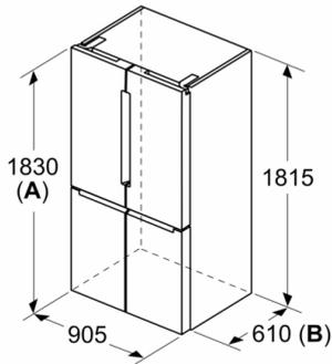
**A:** Front is adjustable from 1830 to 1847, with front levelling feet fully extended
