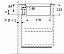
When installing directly against outer walls that are not insulated ( $\mu \geq 0.5 \text{ W/m}^2\text{°C}$ ), we recommend using partially or fully ducted recirculation configurations.
