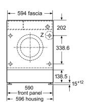
measurements in mm
