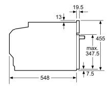
measurements in mm
