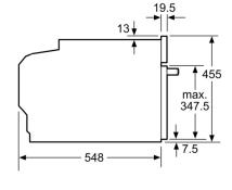
measurements in mm
