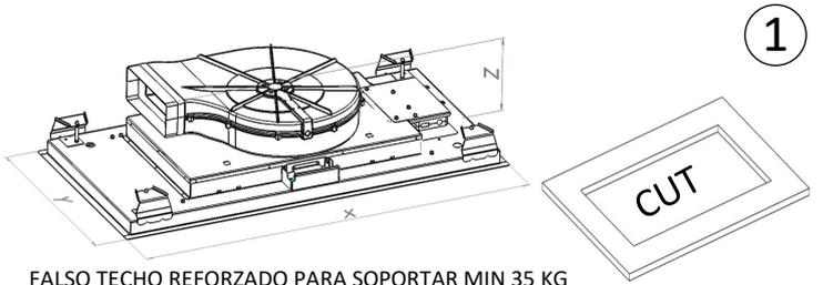
FALSO TECHO REFORZADO PARA SOPORTAR MIN 35 KG
