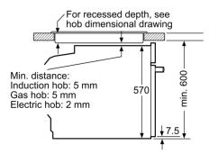
measurements in mm
