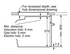
measurements in mm
