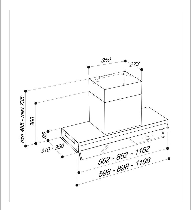
To be installed in a cabinet without base
