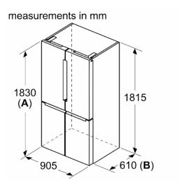
A: Front is adjustable from 1830 to 1847, with front levelling feet fully extendedB: Add 25 for fixed spacers on back
