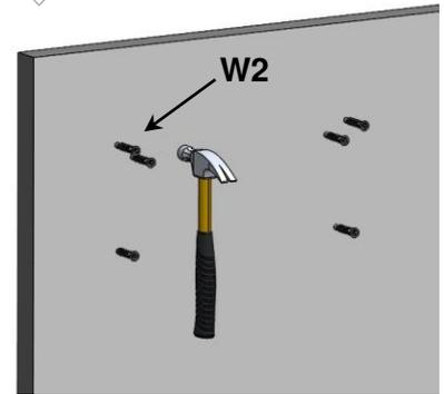
The anchor must be sunk at least 3/8"/10 mm into the plaster coating.
