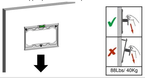
6 Connect the TV to the wall plate by hooking the upper part of the vertical rails on the wall plate
