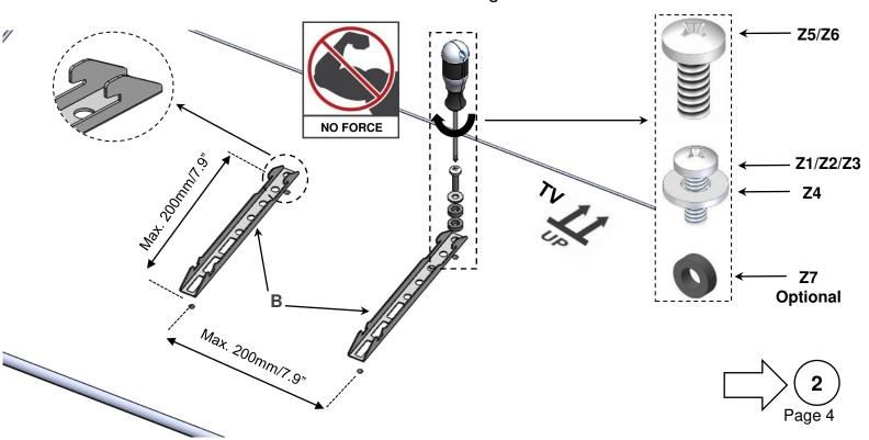
Connect the TV rails (B) to the back of TV at all 4 connection holes, while placing the plastic spacers (Z7) between the TV rails (B) and the back of the TV. Choose the screw that fits the TV's mounting holes diameter.
