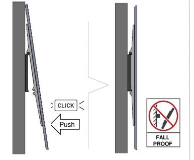
8 Test if the auto-lock mechanism is functioning.
