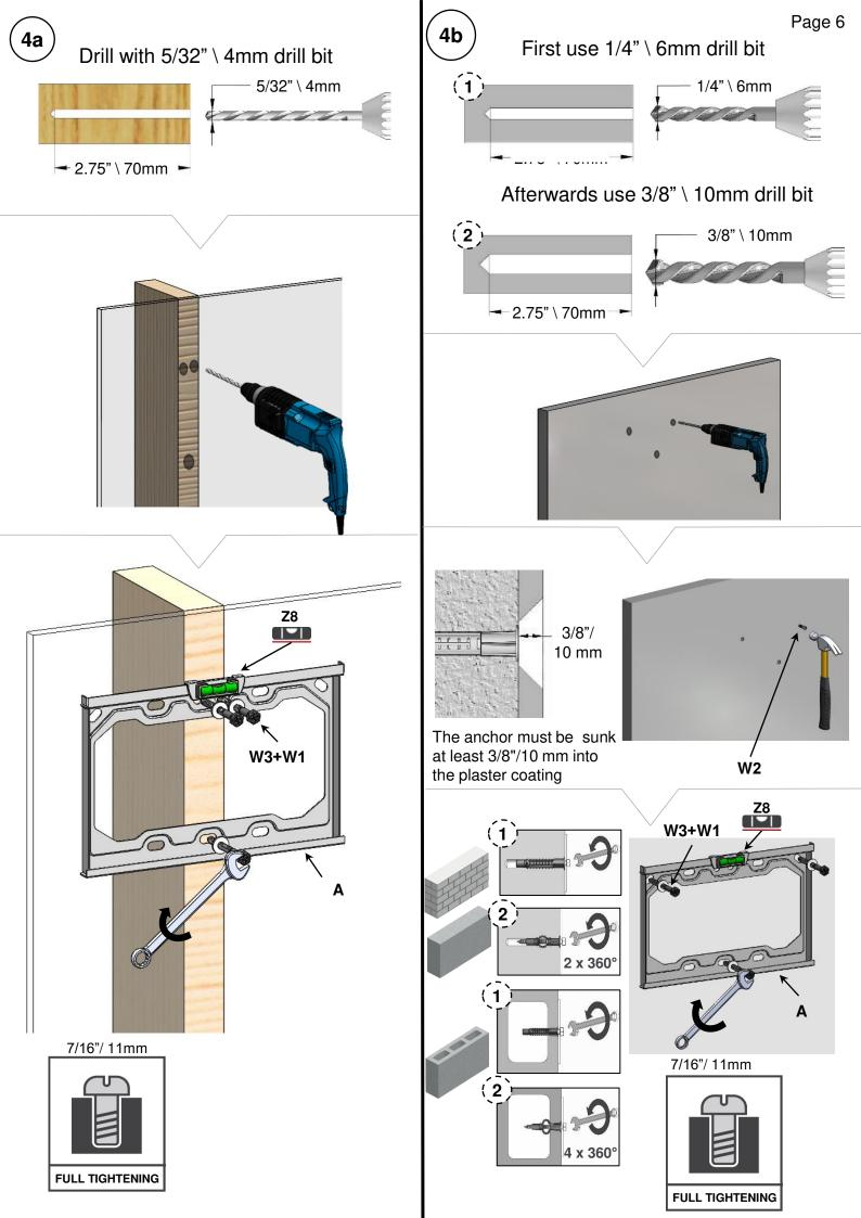
Apply force on the upper part of the Wall plate and make sure it is well connected
