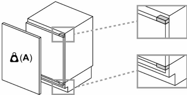
Fitted unit fronts that exceed the permissible weight may cause damage and result in functional impairment of the hinges
