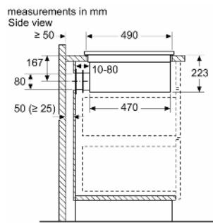
When installing directly against outer walls that are not insulated ( $\lambda \geq 0.5 \text{ W/m}^2 \text{ °C}$ ), we recommend using partially or fully ducted recirculation configurations.
