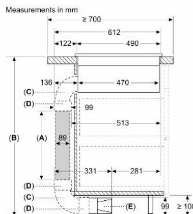
The installer has to select the tube length and if necessary cut it according to the kitchen height
