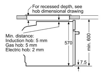
measurements in mm
