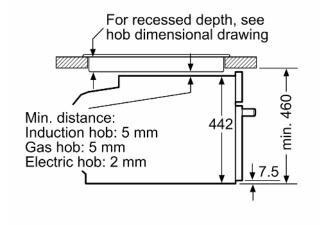
measurements in mm
